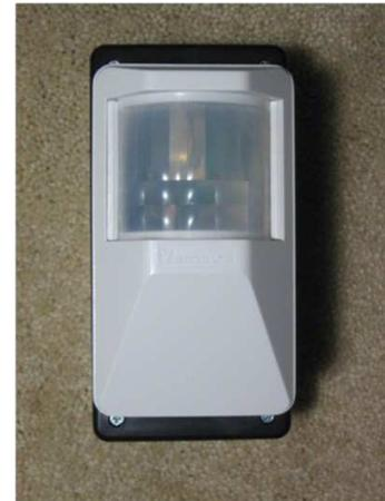
Figure 1: Motion Sensor and Data Logger Unit
