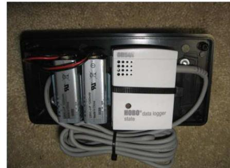
Figure 2: Data Logger and Sensor Battery Setup
