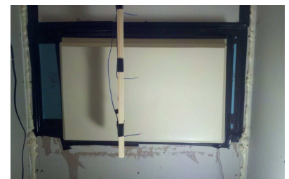
Figure 2: AC sleeve in test lab with rigid indoor cover.
