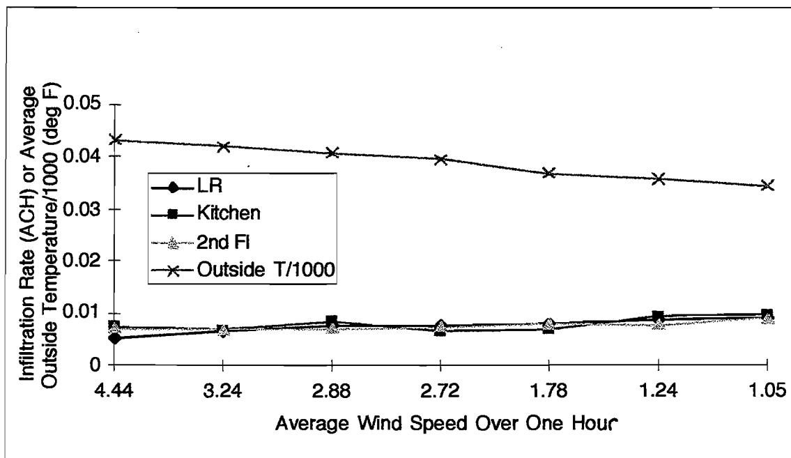
**Infiltration Rate and Wind Speed: Night of 12/19-12/20**
