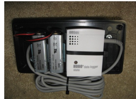
Figure 2: Data Logger and Sensor Battery Setup
