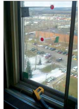
High-rise window example of temperature targets—IR thermometer in foreground.
