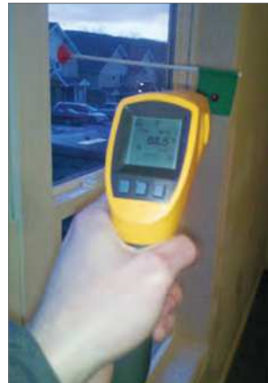
Measuring indoor air temperature with a window-mounted temperature target.
