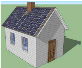
Figure 10 Chimney Obstructs One Panel on a Gable Roof
