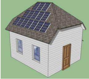
Figure 11 Angles Prevent Panels Filling a Hip Roof
