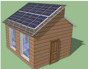
Figure 13 High Receptivity Due to Large South Roof and Small North Roof
