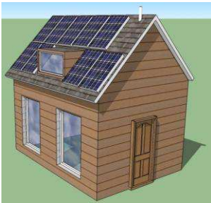
Figure 14 Dormer, Plumbing Vent, and North Roof Result in Low Receptivity
