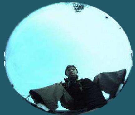
Nick Kirk uses a fisheye lens to check out the solar access of a potential residential rooftop installation
